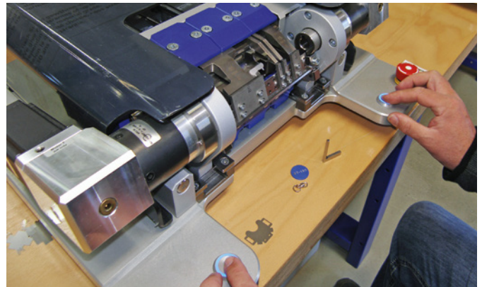
Since the eight stepper motors in the BT-150 are controlled by four 2-axis ACOPOSmicro modules, there is no longer a need for homing after a disruption or product changeover. (Photo: Franz Rossmann)
